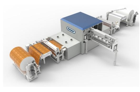
here, is the next 'Planet' - we call it 'SATURN'. So, the Hymmen SATURN Digital Printing Line is our new development with water-based inks for decor paper. It can be used for producing decor paper at the customers' site. Then this paper can be impregnated and e.g. used in short cycle presses for furniture, for flooring and other applications.
