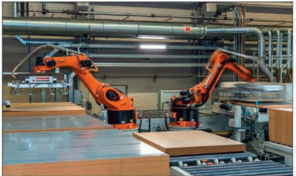
Feeding the CCI line at Egger in Brilon with robots (photo courtesy of Egger)
