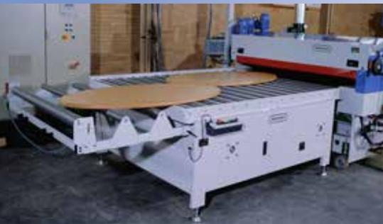
feeding rake for different workpieces
