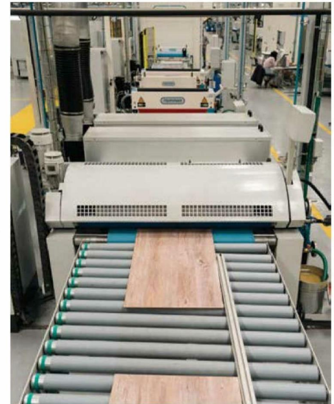
The Hymmen technology – Digital Lacquer Embossing (DLEplus) – details of the production process at Amorim (Copyright Amorim)
