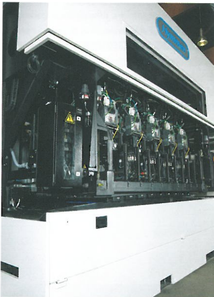
Figure 5: The core of Hymmen's digital printing know-how is in the ink units
