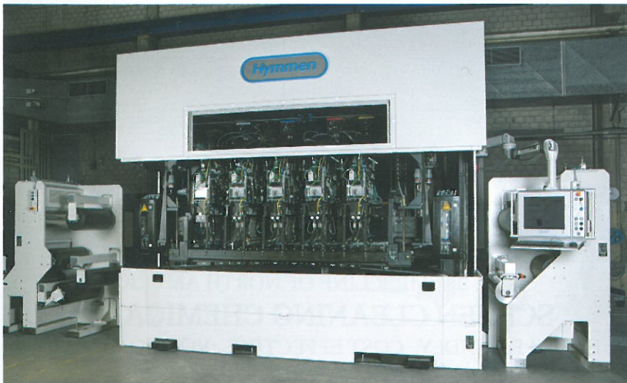
Figure 1: showing cover closed (top) and cover open on the digital edge printing line Jupiter JPT-WS as a compact whole unit
