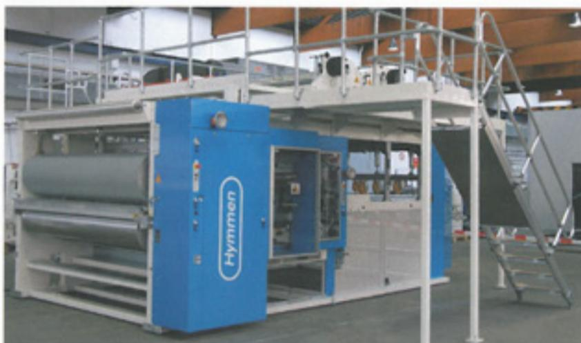
Fig. 3: One of four Laminating Lines sold by Hymmen this year: CTK with rubber calender for laminating special foils.
