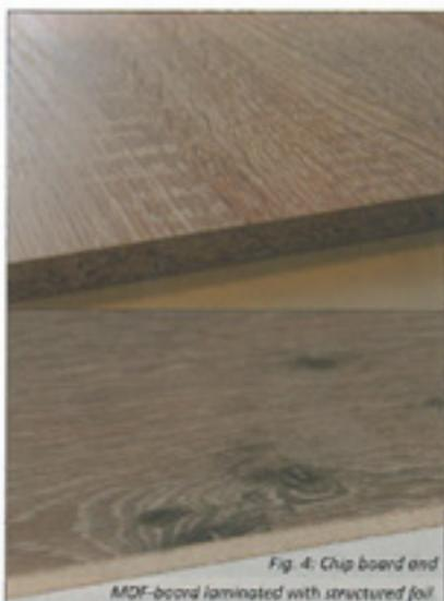
Fig. 4: Chip board and MDF-board laminated with structured foil.
