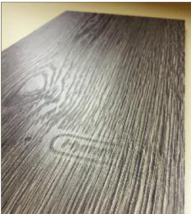
*With a width from 70mm up to 2.100mm the technology can be integrated into exiting process chains easily. By only using a small amount of the structuring medium all proven features like hardness, bonding, resistance and chemical reliability of the core lacquer are assured. Last but not least certainly it is possible to create structures that are embossed in register (EIR) to the decor of the surface - no matter if printed digitally or analog.*
